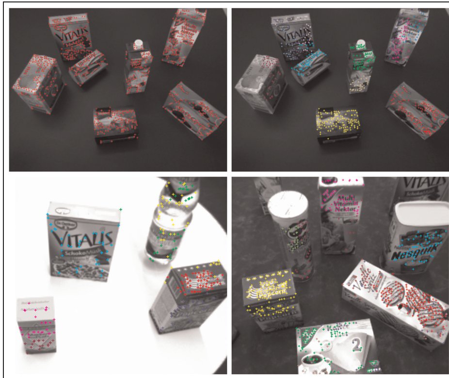
Figure 4. Initial object hypothesis generation. In the top row, the left image shows all three-dimensional points resulting from the stereo matching of Harris interest points and color MSERs. The right image depicts the object hypotheses that were generated from these points. The extracted features are shown with differently colored crosses to indicate which of the hypotheses they belong to. The bottom row shows the initial hypotheses that were generated for two different settings. Objects are well separated in the left image scene, hence it is relatively easy to create object hypotheses. If the scene is as cluttered as in the right image, purely vision-based approaches reach their limits and hypotheses become more likely to include features from different objects.
