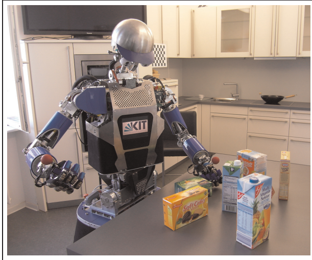
Figure 3. The humanoid robot ARMAR-III interactively discovers objects that can typically be found in a kitchen environment, segments them and learns their visual appearance.
