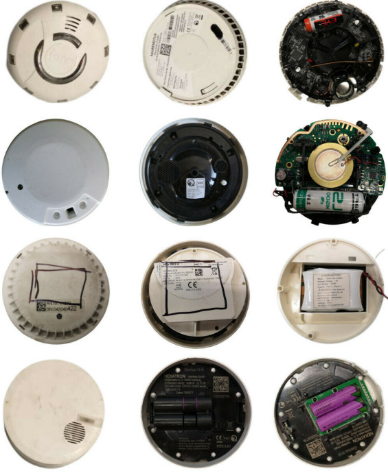
Fig. 8. Front, back and internal views of different smoke detectors.
