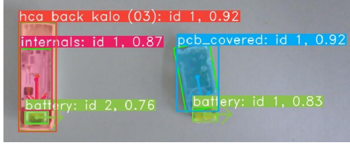
Fig. 2. Identification and localization of different devices based on instance segmentation.
