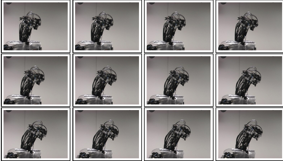
Fig. 2. DB pursuing the toy dog. These images illustrate that the head (3 DOFs) and the torso (3 DOFs) of the robot also move to support the pan and tilt motion of the eyes (4 DOFs), which are primarily responsible for getting the object in the fovea.
