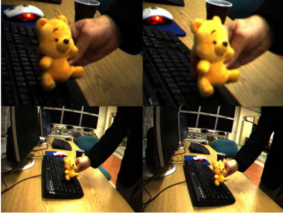
Fig. 6: Simultaneous stereo view from peripheral (below) and foveal cameras (above)
