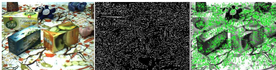
Fig. 1: Segmentation of unknown objects. Original image (640x480) on the left, extracted edges (Canny edge detector, threshold 0.01) in the middle, and extracted SIFT features on the right.
