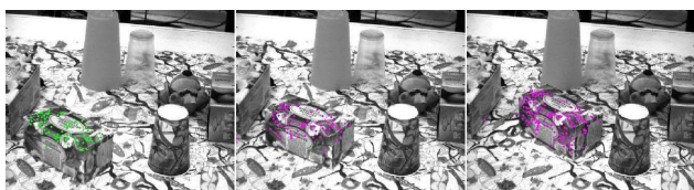
Fig. 9: Building object model. Hypothesis (left) with object features after first push (middle) and after second push (right).
