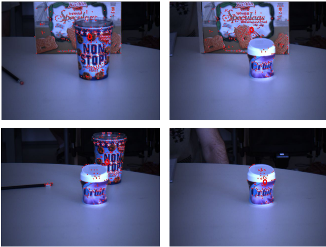
Fig. 5. Recognition of initial hypotheses in the foveal view depends greatly on the amount of features in the background. In the upper left image we have an unknown object in the background, but the object in the foreground is correctly recognized, since it is very rich with features. In the upper right image the object in the foreground has much fewer features and is therefore incorrectly recognized. For the same reason, the object in the lower left image is falsely recognized as the known object in the background. If there are few features in the background, as seen in the lower right image, the recognition of objects in the initial hypotheses can reach 93%.
