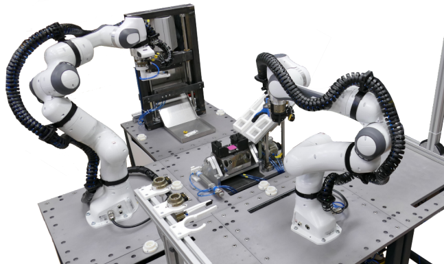
Fig. 1. Reconfigurable robotic workcell for automated recycling of electronic waste. The targeted recycling procedure involves the disassembly of electronic devices to remove batteries.
