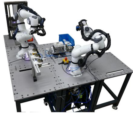
Fig. 1: An example of a robotic workcell used for recycling of waste electronics, built using our modular robotic workcell platform.
