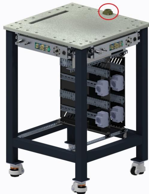
Fig. 2: 3D render of the archetypical module, with a quick calibration feature circled in red.
