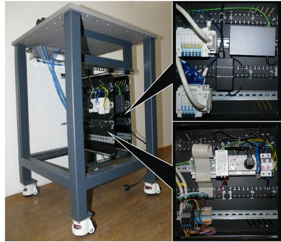
Fig. 3: Electronics of an archetypical module mounted on pull out panels.
