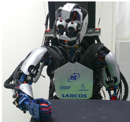
Fig. 1. Humanoid robot CB-i touching an object placed on the table. It has an active visual system, which on the one hand improves the object fixation capabilities, but on the other hand reduces the accuracy of 3-D vision.
