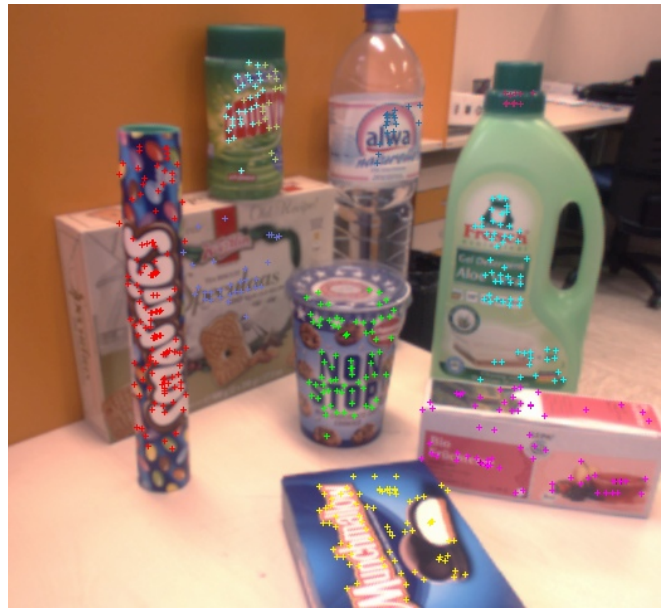
Fig. 3. Initial hypotheses that were generated for a number of typical household objects. Crosses of the same color belong to the same hypothesis.
