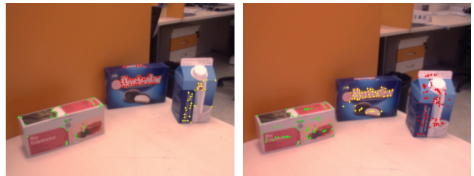
Fig. 4. The left image shows hypotheses generated using only Harris interest points. In the right image, color MSERs are used in addition to them, which enables us to recover the surfaces more completely.
