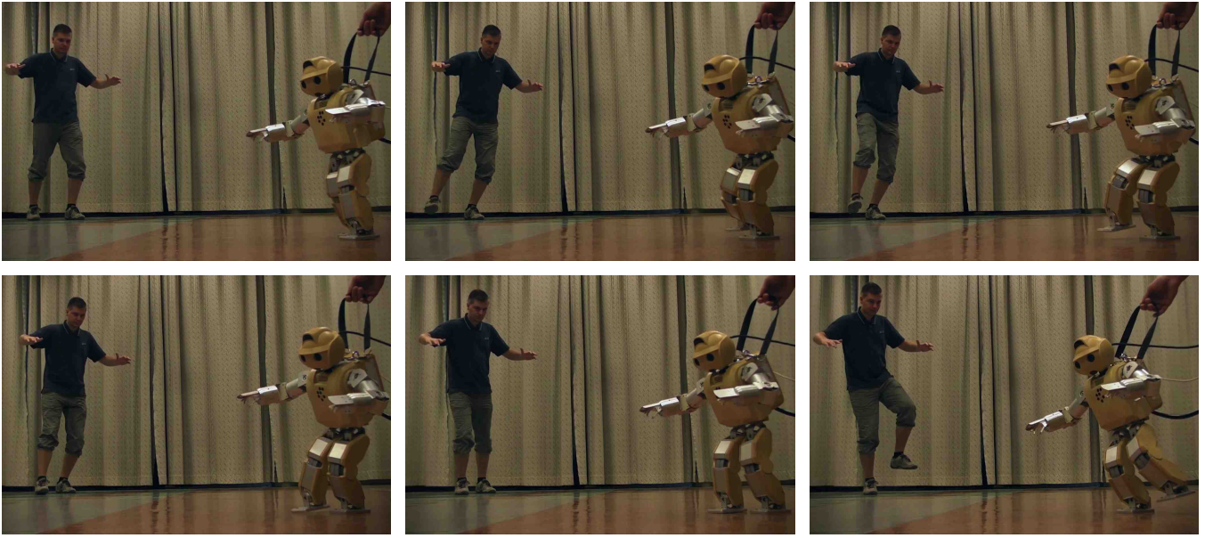
Fig. 2. Real-time transfer of a walking movement.
