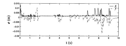
Fig. 6. TCP tracking error.
