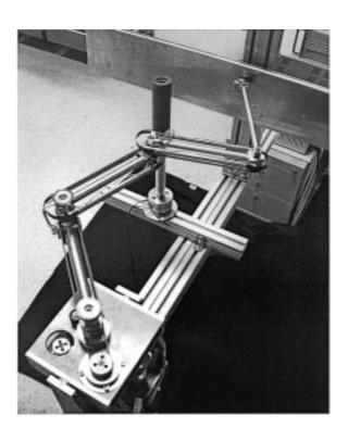
Fig. 1. 4-DOF experimental robot.
