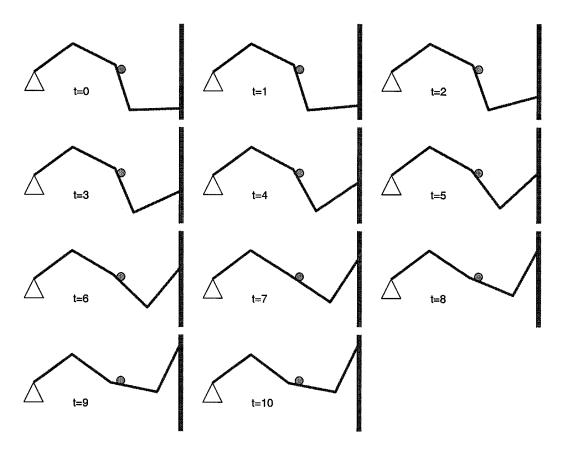
Fig. 5. Poses of the robot during the simulation of the task.
