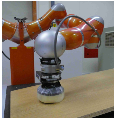
Fig. 1: Experimental setup for the evaluation. Non-rigid contact, i.e., wiping of surface was chosen as the use-case scenario. The robot adapts its motion based on the observed passivity.
