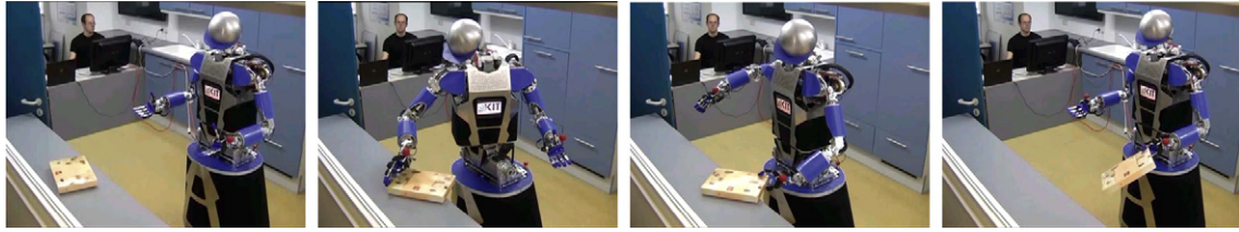
Fig. 11. Execution of the plan involving the OACs PlanPush , AgnoPush , PlanGrasp , and ObjGrasp . From left to right: (1) the object is not graspable, (2) pushing moves the object into a graspable pose, (3) the object is grasped, and (4) the object can finally be picked up by the agent.
