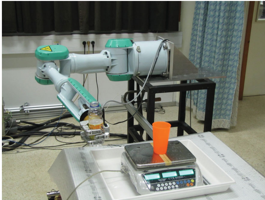
Fig. 3. (Colour online) Experimental setup for pouring.
