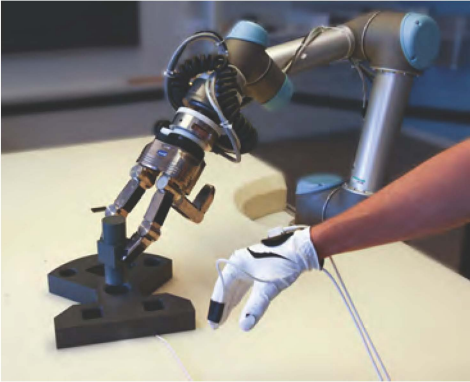
Fig. 2. The tele-operating setup with the hand-mounted sensor and the Universal Robots arm.
